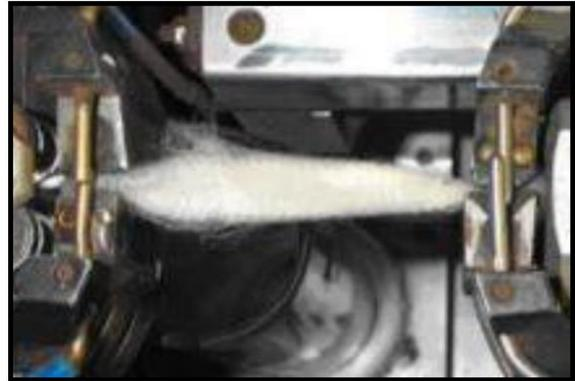
Fig 2: A Staple about to be broken in the ATLAS jaws
