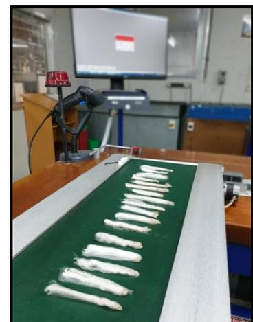
Fig 1: A series of staples prepared for length and strength measurement
