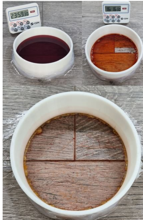
Figure 2: Pooled liquid over a “T” joint with time lapse
